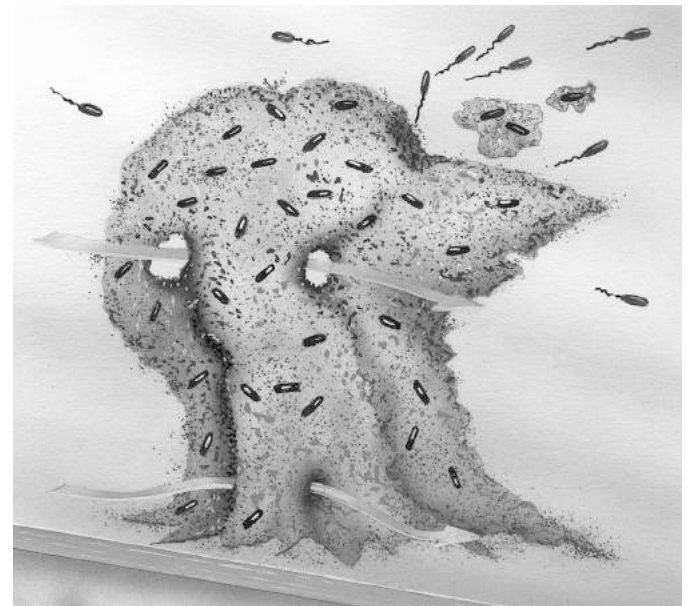
Figure 7. Massive biofilm tower becomes extremely resistant to attack by cleaners, disinfectants and antibiotics. Pioneer organisms and pieces of biofilm break loose and flow to other locations within the system.
